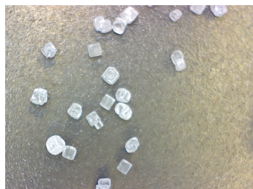
An image of multiple salt crystals viewed through a USB microscope. The crystals have a clear cubic structure, and are all roughly the same size (there is some variation).
